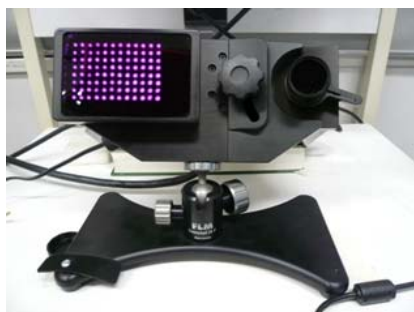
Figure.1 アイカメラ (EyeLink SR Research 社製)
